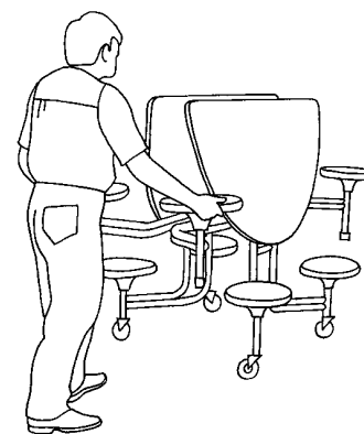
GRASP BOTH MIDDLE STOOLS AND PUSH TOGETHER TO ENGAGE LOCK.
