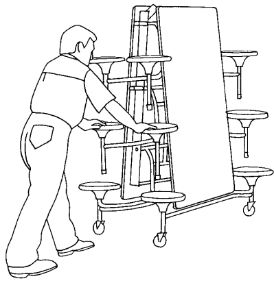
PUSH FROM END OF TABLE WITH TRANSIT LOCK ENGAGED.
